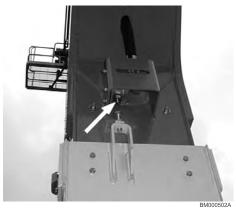
Figure 4. Tower Boom Horizontal Limit Switch
