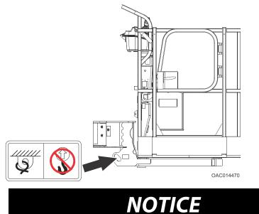
Secure turntable with turntable lock (if equipped) before traveling long distances or hauling machine on truck/trailer.
