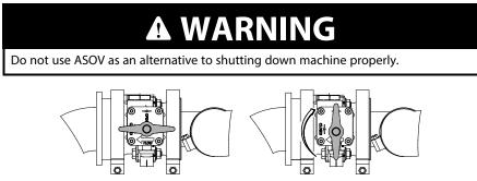
Figure 9. ASOV Reset (Closed to Open Position)
