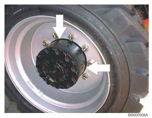
Lube Point(s) - Level/Fill Plug Capacity - 17 oz (0.5 L) - 1/2 Full Lube - EPGL
