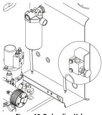
Figure 12. Re-leveling Valve
