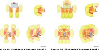
Figure 35. SkySense Coverage Level 1 Areas (2– Bar)
