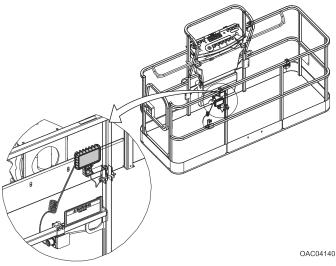
Figure 30. Portable Work Light
