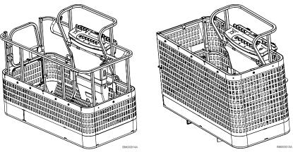
Figure 23. Fabric Mesh to Mid Rail
