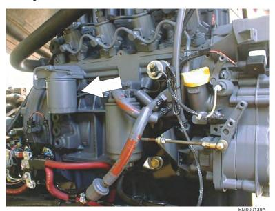
Lube Point(s) - Fill Cap/Spin-on Element Capacity - 11 qt (10.5 L) Crankcase; 5 Quarts Cooler Lube - EO Interval - Every Year or 1200 hours of operation Comments - Check level daily/Change in accordance with engine manual.
