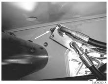
Figure 3. Tower Boom Vertical Limit Switch
