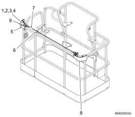
Figure 20. Bolt-On External Fall Arrest System
