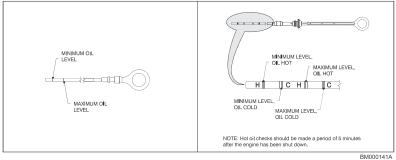
Figure 45. Deutz 2011 Engine Dipstick
