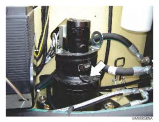
Lube Point(s) - Level/Fill Plug Capacity - 43 oz (1.3 L) Lube - 90w80 Gear Oil Interval - Check level every 3 months or 150 hr of operation; change every 2 years or 1200 hr of operation
