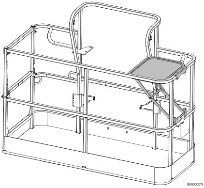
Figure 29. Platform Work Surface
