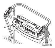
Operator passes through path of sensor beam.
